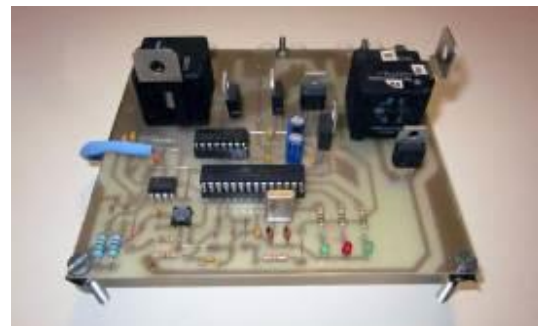
Figure 14. Battery charger PCB.
