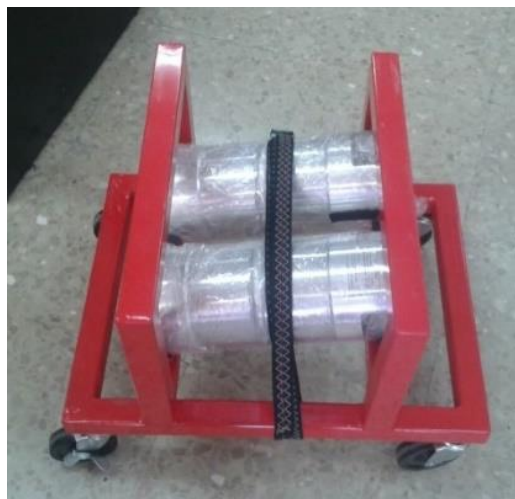
Figure 26. Hydrogen storage metal hydride cylinders for testing in UHU.
