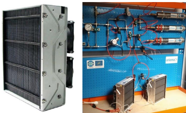
Figure 30. Fuel cell stacks in AQUASEF's system Left: view of the selected fuel cell stack. Right: picture of the two stacks integrated in the final system.
