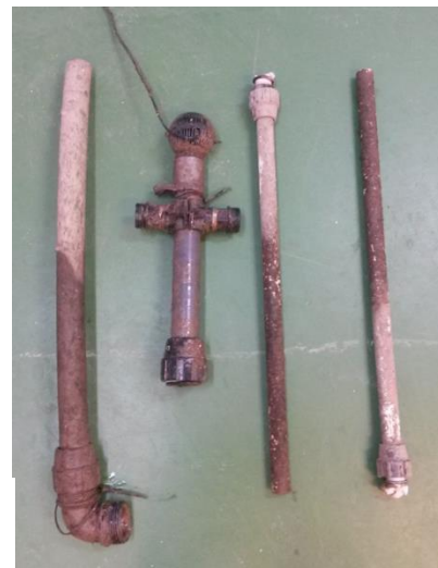
Figure 37. Materials tested in the study for avoiding deposition and fouling on the pipes and pumps
