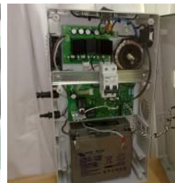
Figure 18. General vision of the first Plug & Play PV compact.
