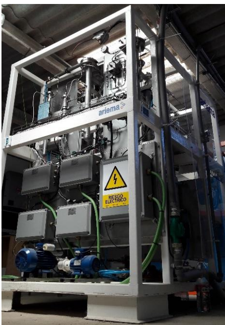
Figure 24. Steps for the electrolysis prototype's activity: design and 3D drawing (top left), transport and installation (bottom left), final placement and testing (right).
