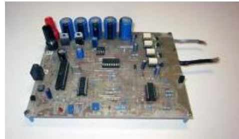
Figure 15. Full Inverter PCB. All components were integrated
