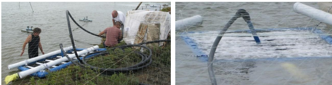
Figure 36. The second diffuser (definitive prototype) being placed in an open pond. Right: The same diffuser just before sinking to its final position. Bubbles already being generated
