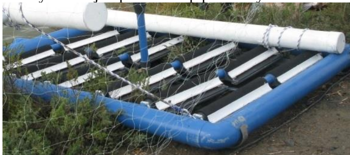
Figure 33. Left: O2BTech with its 12 diffusers and two floats. Right: the MicroBTech being tested in the laboratory
