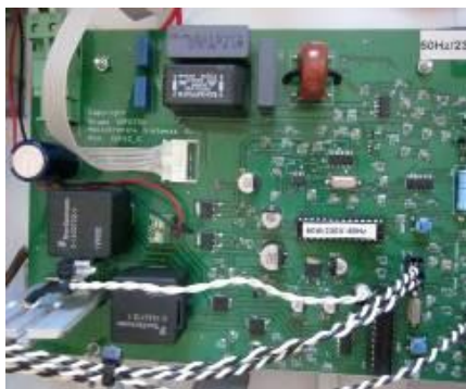
Figure 16. Inverter without Power transistors and Battery load regulator PCB.
